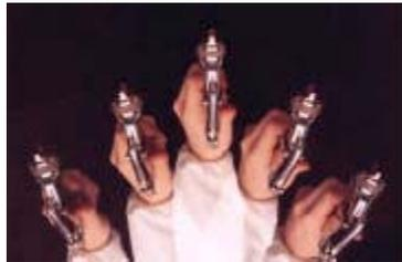
Arcing the gun causes uneven paint distribution
