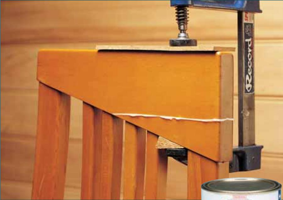
Two-pot high strength gap filling adhesive.
