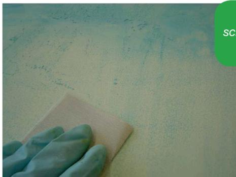
***Sanding Guide Coat** assists in making fine scratches appear as easily visible blue lines that can be sanded away as you progress*
